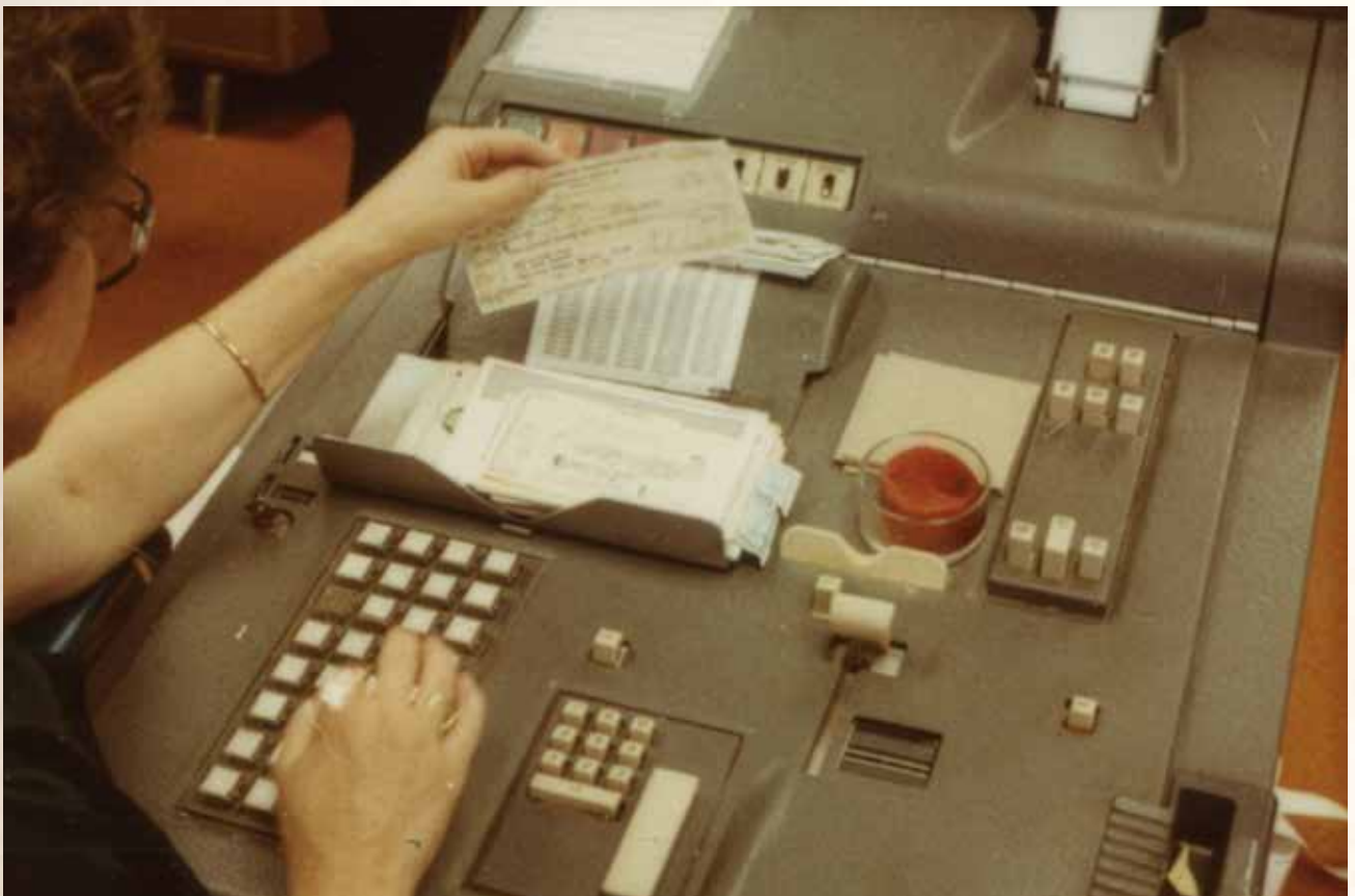
An employee loads checks into an IBM 3890 high-speed sorter. These machines could process 2,400 checks per minute.
