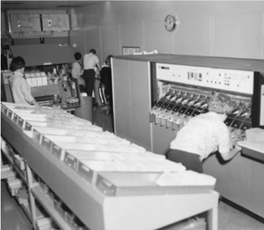
Workers at the Omaha Branch of the Kansas City Fed in the mid-1960s use a high-speed check reader produced by IBM.
